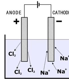
Fig. 7. The movement of charged NaCl particles in solution
