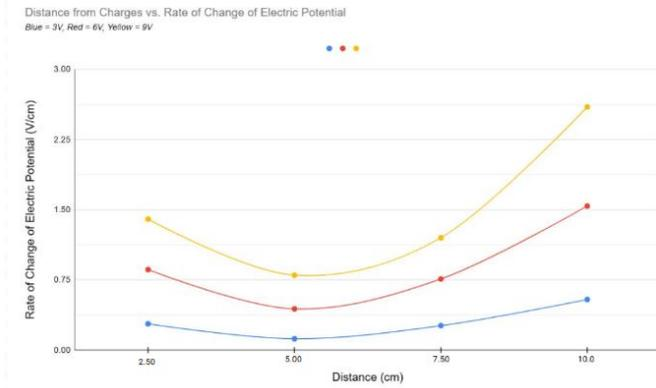
Table 1/Figure 6: Table and line graph model of the points along each path, with their distance from the cathode from the charges (measured in centimeters) and the rate of change in electric potential between each increment (measured in volts per centimeter) displayed
