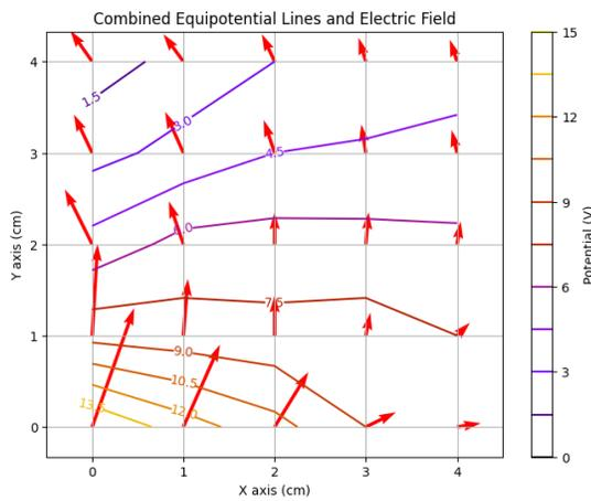
Fig. 6. The equipotential and electric field lines
