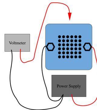
Fig. 1. Diagram of the experimental setup. Measurements were taken in a 3-cup polypropylene food storage container with a pre-marked 6 cm x 6 cm grid. The container was energized using negative and positive electrodes connected to a power supply. For each point, potential difference was measured with respect to the negative electrode.
