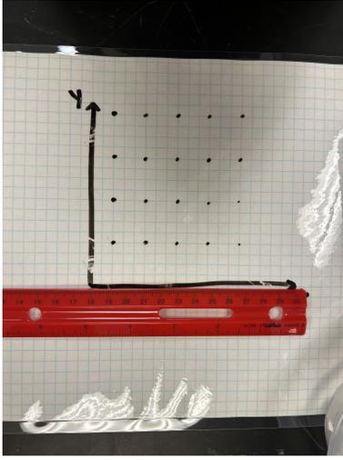
Fig. 1. The grid of points. Each square is 0.25 inch (0.635 cm). Measurement grid points are 3 grid squares (1.905 cm) in  $x$  and 4 grid squares (2.54 cm) in  $y$ .
