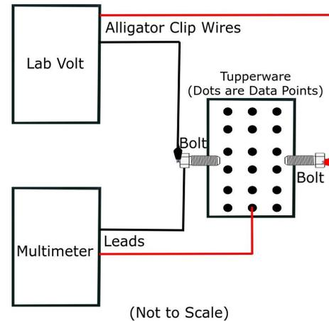
Fig. 1. The experimental setup consisted of a small polypropylene container containing a saline solution, positive and negative electrodes, and a grid marking the  $6 \times 3$  array of test points to be measured. The system was energized with a Labvolt 197P power supply set to 3.7 V. Measurements of the potential between each point and the negative electrode were made using a digital multimeter.
