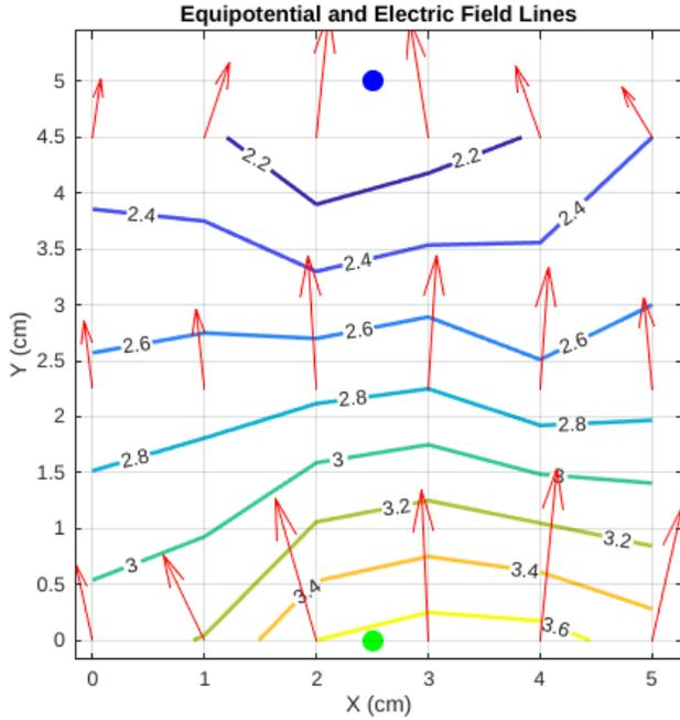
Fig. 2. Results of Table I plotted. Positive electrode shown as green dot (bottom); negative electrode shown as blue dot (top). Equipotential lines labeled with the potential value in V; electric field lines shown as red arrows.
